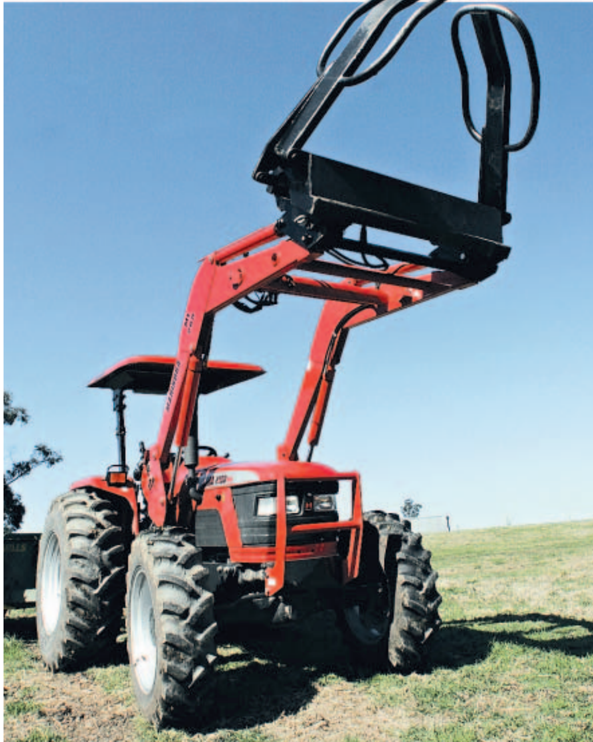
More power: a bale clamp takes full advantage of the Mahindra's front-end loader. Pictures: MARK GRIFFIN
